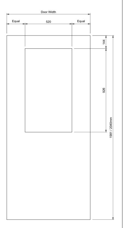
Description: Doorpac Standard Aperture - 8G - 508 x 914mm - 150mm Top Margin & Centred In Width - FD30/30 & FD60/60 Machining
